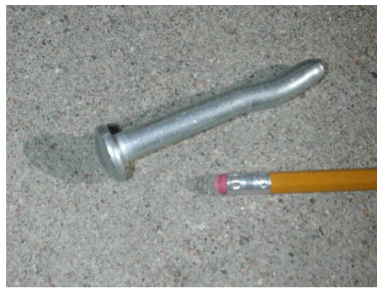
Detail of the vandal resistant fastener – Rawlplug #5550 (photo courtesy James Mackay, City of Denver)
